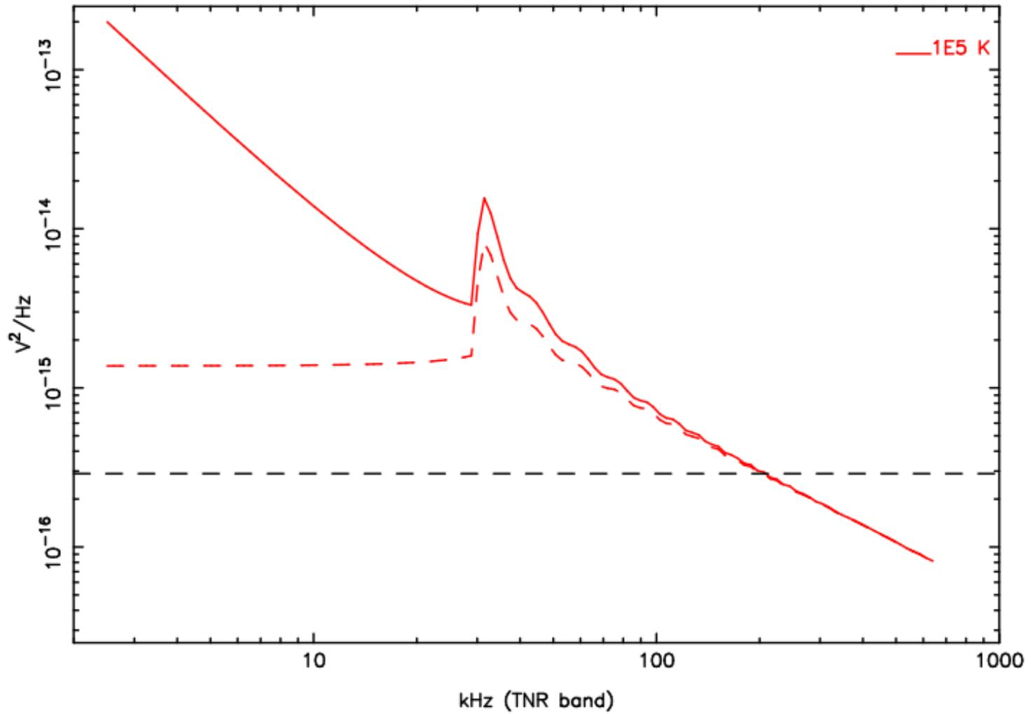
QTN power spectra samples on PANT (fp=30kHz)
