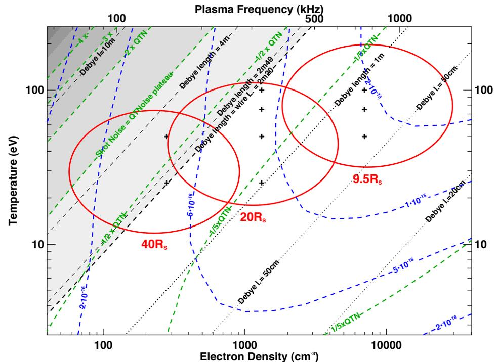
QTN power spectra samples on FIELDS/SP+ ( $f_p=150,325,750\text{kHz}$ )
